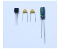
Push the voltage regulator in the IC1 position, right next to the switch. Bend the leads to fit it into the holes. Look at the white contour printed on the PCB for polarity; the chamfered side of the voltage regulator should line up with the line on the board, and the rounded side with the half circle. Push it far enough to have an equal length of leads on either side of the board, i.e. push it in
