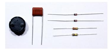
Almost there! Install the buzzer at position X1 and solder it in place. It doesn't have a polarity, so can be oriented either way. Continue with the 22 nF capacitor, a large brown capacitor that fits in position C10. Check its value, it should have the text "223" printed on it. Solder it in place as well. Like the buzzer, it doesn't have a polarity. Finish with the diodes in positions D3 and D4, and the resistors of 100k and 22k in positions R6 and R14 respectively. Clip the leads short.
