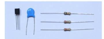
Solder a second 2N3904 transistor in position Q3, as with Q2 before. Proceed with the 330 pF capacitor, easily recognisable by its bright blue package. This capacitor doesn't have a polarity and can be installed in either orientation in position C8. Finish up wih the resistors in positions R9, R12, and R4, and trim leads.
