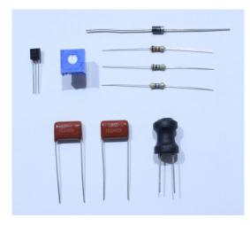
Switching current through an inductor will cause the voltage to spike, and that effect is used here to generate a high bias voltage for the SBM-20 Geiger tube.
