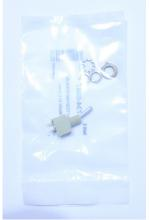
Open the bag containing the switch and discard washers and nuts – these won't be needed. Push the switch in position next to the battery holder. It can be installed in either direction so don't worry about polarity. Solder the 2 electrical contacts of the switch, making sure the switch is flush with the PCB. Ask someone else to hold the switch in place if necessary.
