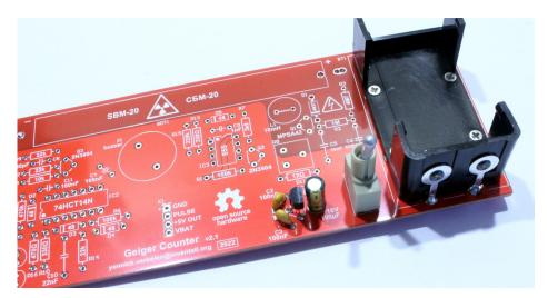
**4. Power LED** Components: 470Ω resistor, green LED
