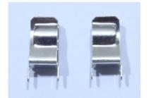
At either end of the GM tube place holder at the top of the board, install a tube socket. Each socket has a "notch" that stops tubes from falling out sideways, so make sure to orient the sockets such that these notches are oriented outward.
